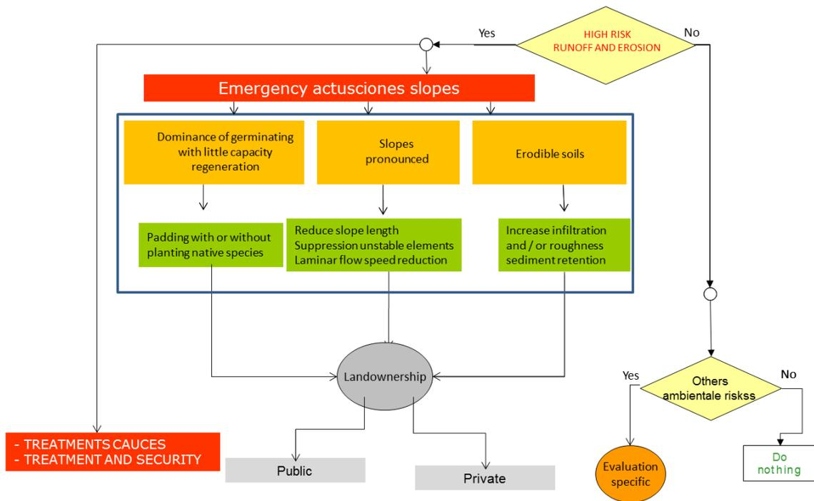
Figure III-24. Diagram of support to decision-making process to assess the need to apply emergency actions to fight erosion in hillsides.
