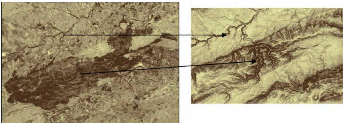
**Figure 15.** Left: distribution of the dNBR index over the whole image analysed (higher severity based on the colour intensity). Right: Digital elevation model. The arrows indicate the riverbed of Clariano river and the Barranc dels Tarongers. As in the Barranc dels Tarongers, the values of the dNBR index in the riverbed of Clariano river are high, which may be due to the different phenological state of the riverside vegetation, the presence of water bodies and the terrain features.
