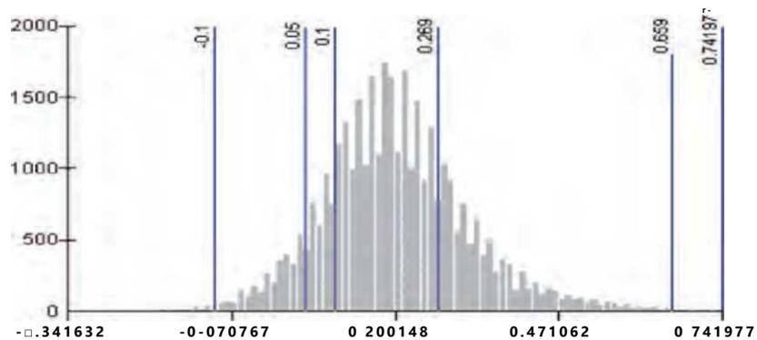
**Figure 14.** Histogram with the distribution of the dNBR index in the pixels included in the burned area. Most of them (75%) present values lower than the threshold 0,269, which is deemed as the limit for low severity. Almost 10% would be included in the 0.05-0.1 interval that, according to the scale of Key and Benson (2006), would correspond to unburned areas; however, they correspond to low severity areas. In Chart 4, the values of the index have been multiplied by 1000.
