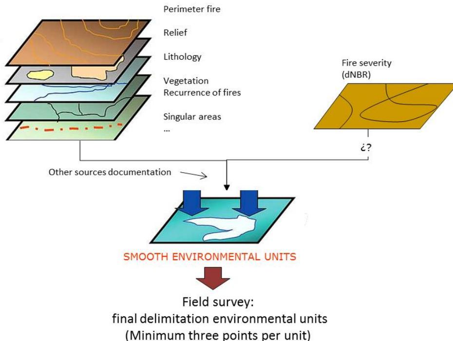
**Figure III-4.** The division into environmental units is carried out firstly using the cartographic information available and it is adjusted later according to the information obtained during the area inspection.
