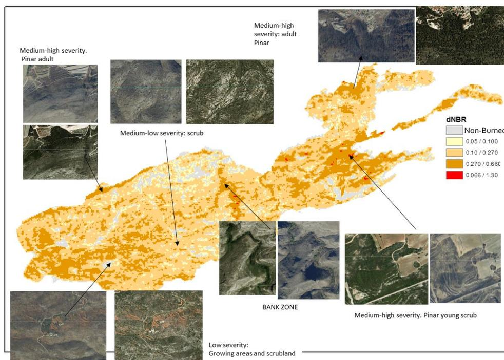
**Figure 13.** Distribution of the severity intervals obtained with the dNBR index. The images reflect the situation before and after the fire (based on ortophotos of 2009 and 2010). Key: Grey: unburned. Yellow: dNBR 0.05-0.10. Light orange: dNBR 0.10-0.270. Dark orange: dNBR 0.270-0.66. Red: dNBR 0.66-1.30.
