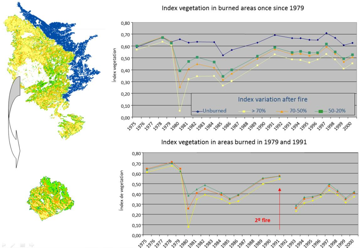
**Figure V-1.** Evolution of natural regeneration on the forest surface affected by the Ayora fire in 1979, analysed as per a vegetation index obtained through Landsat images during the 1975-2001 period. Top: burned surface once since 1979. Bottom: burned surface in 1979 and 1991.
