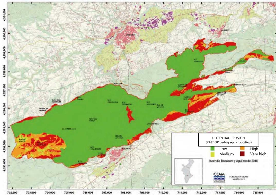
Figure 4. Potential erosion (PATFOR cartography modified by lithology). Key: Green: low. Yellow: medium. Orange: high. Red: very high.
