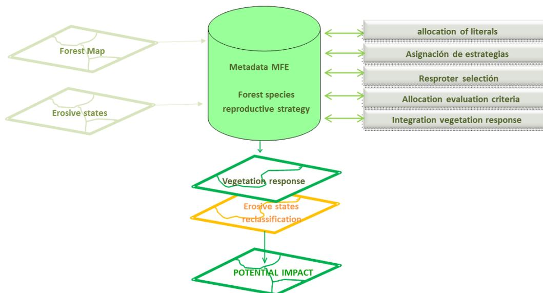
**Figure II-6.** Cartographic information, forest maps and cartography on soil erosion are processed within a GIS environment where reproductive strategies are assigned (the total canopy cover fraction occupied by resprouters is calculated), as well as re-classifications and overlaps.
