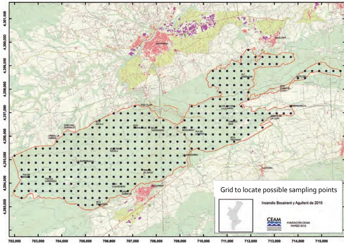
**Figure 11.** Theoretical distribution of the sampling points according to the predefined mesh. A total of 25 points (11 sampling points and 14 observation points) were subject to inspection.
